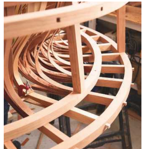
The build called for many mortise & tenons
